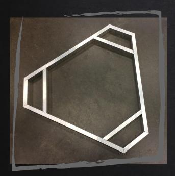
Is a version of a "holonomic drive," essentially meaning there is no defined forward direction Use 3 gearboxes and 3 omni wheels Can be built without using any chains or belts Making sure the wheels are in the same plane isn't an issue with Kiwi drives, Can be made to be much more user friendly through the use of sensors like gyros and encoders
