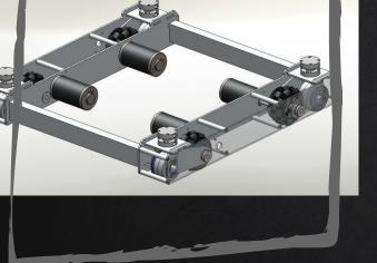
Uses 4 "butterfly modules" at each corner of the robot with 2 wheels each
