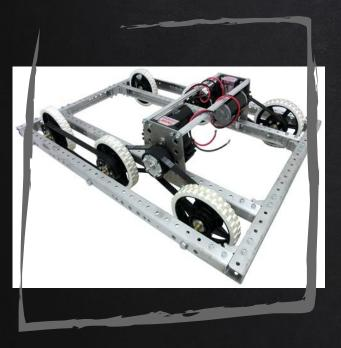
Includes West Coast Drive, 6WD Tank, 8WD Tank Uses a skid steering and traction wheels powered by 2–6 motors Many different things to do with tank drives:
