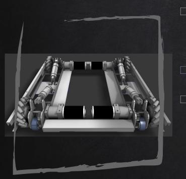
Same thing as butterfly except replacing the omni wheels with mecanum wheels
