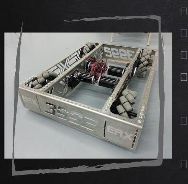
The second most common drivetrain in FRC Pronunciation: Meck-an-um Spelling: Mecanum (no "h") Uses specialized wheels with rollers all around the wheel mounted at 45 degree angles to strafe Each wheel must be controlled by an independent gearbox (4 motors and 4 gearboxes required) Mecanum drives are often made better by using sensors like gyros and encoders
