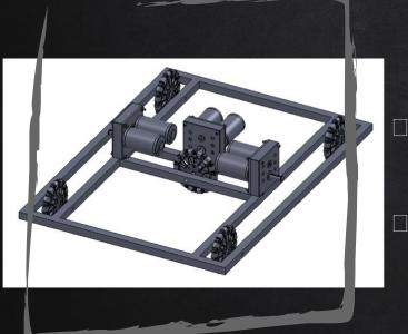
Essentially a tank drive with omni wheels replacing traction wheels and an extra omni wheel and gearbox mounted perpendicular for strafing Has the same maneuverability as mecanum with less gearboxes The strafe wheel can be difficult to mount - needs to be near the center of gravity, and getting the
