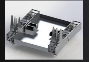
Same thing as butterfly drive except it uses just two longer pneumatic cylinders (the back legs of a grasshopper) to actuate from omni to traction mode
